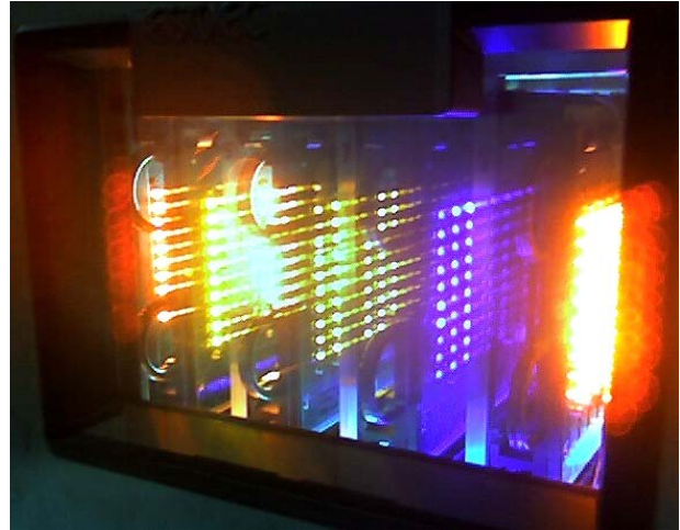
Figure 1: Series Mounted LEDs Undergoing Stress Screening
