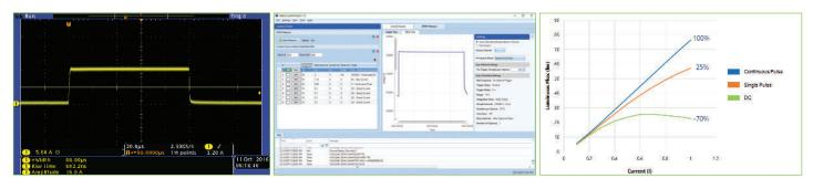
SpikeSafe Precision Pulsed current sources feature precise, accurate triggering and microsecond rise times resulting in square pulses down to 10µs width.
