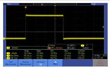
Keithley triggered 15.3ms pulse, 250us jitter
