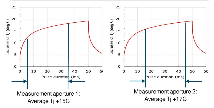
Example: 10ms trigger jitter => 2C difference => 0.4% measurement uncertainty
