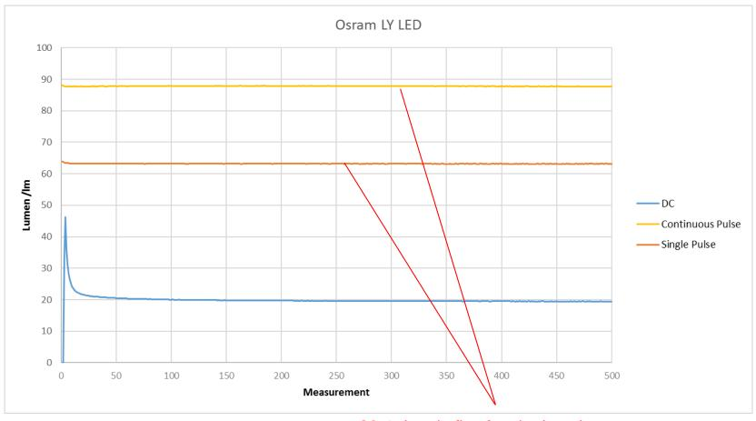
30% drop in flux for single pulse, even with 15ms pulses
