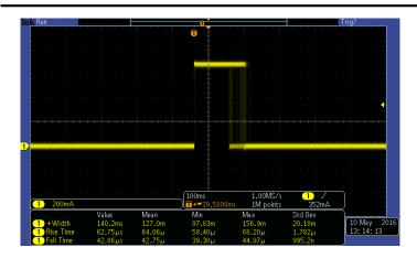
Keithley synchronous mode, 127ms pulse 30ms jitter
