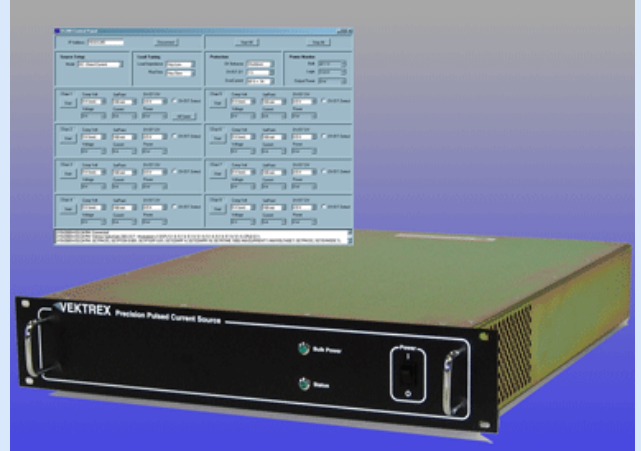
SpikeSafe 200 8 channel for up to 320 5V DUTS
