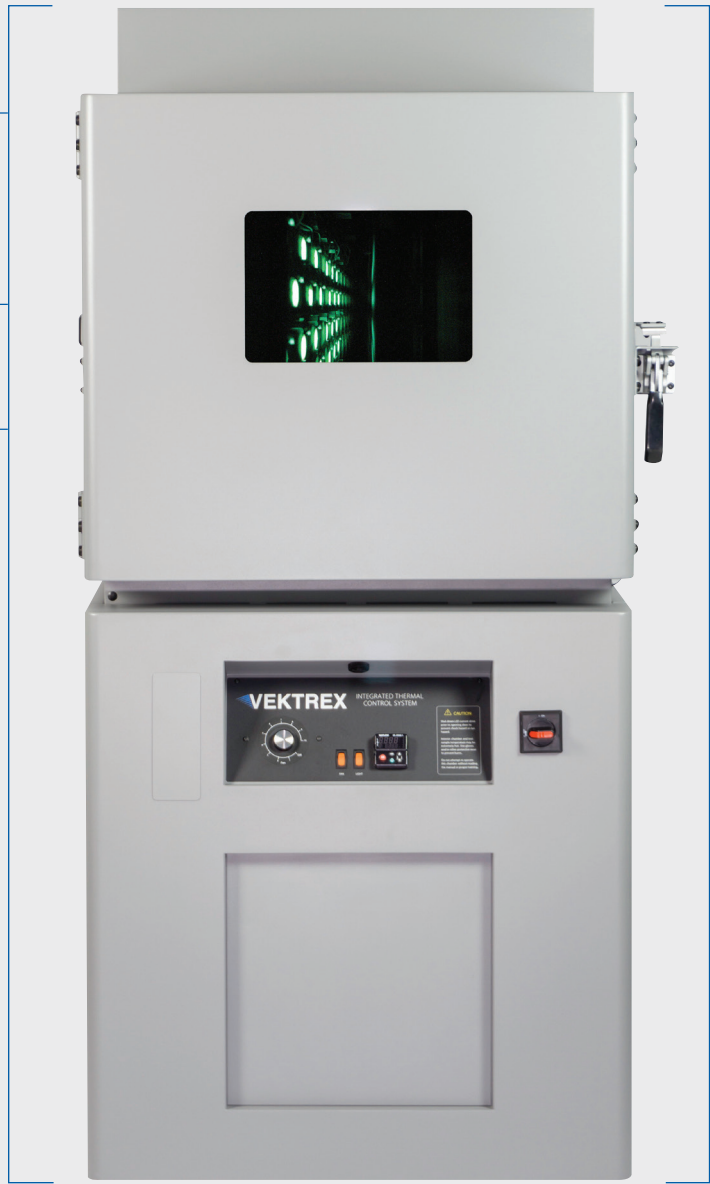
Vektrex ITCS chambers meet LM-80 requirements.
