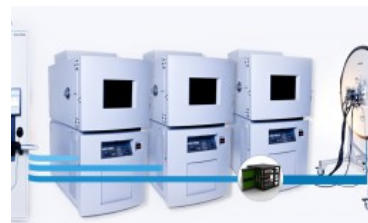
Typical LM-80 System Configured For 3 Temperatures Photo courtesy of Vektrex
