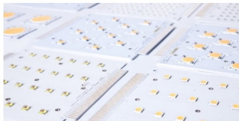
LEDs mounted on test load boards
